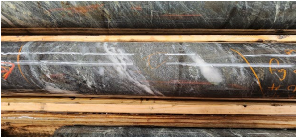
Photo 1: GTCM25-056A at 2706.80 to 2706.95 metres downhole showing chlorite-biotite altered rock with quartz-carbonate veining and fine-grained arsenopyrite and pyrite
