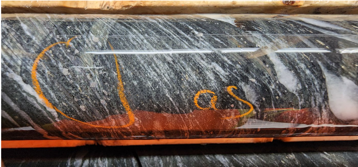
Photo 2: GTCM25-056A at 2695.33 metres downhole showing blocky arsenopyrite along vein margins
