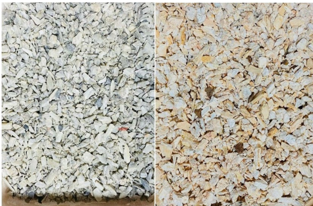
Figure 2: Example images of spodumene concentrate (left) and calcination product (right).
